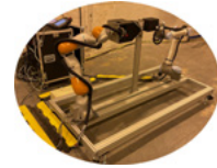
Independent robotic arms either side of the weld building up images for a Computed Tomography (CT) scan
