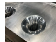
Complex cladding achieved inside nozzle and finish machined
